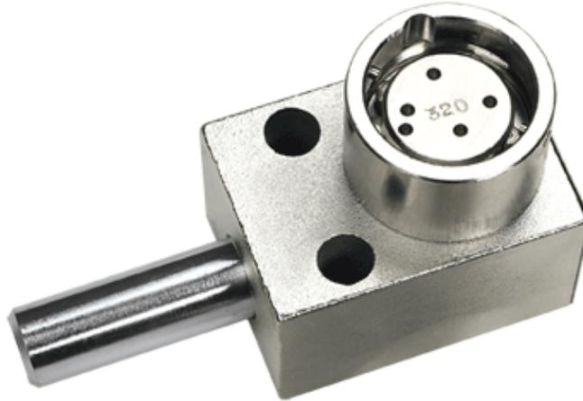
The Type F interlock is generally flat or face mounted with bolts through the front of the housing. Many breaker, switch and T/R manufacturers offer provisions for mounting Type F interlocks.
